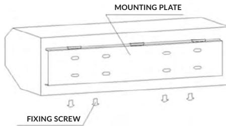
**3.1.2** Fix the bolts in the proper position (decide the position with the mounting plate and pour cement into the bolt holes).
