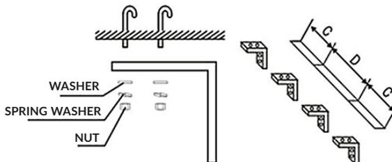
**3.3.3** Set the mounting plate on the ceiling brackets and ensure safe & fixing (use the bolts attached to the ceiling brackets as Fig). Using the ceiling brackets to hang from the ceiling, the position of mounting plate can be adjusted in the limit of 100mm.
