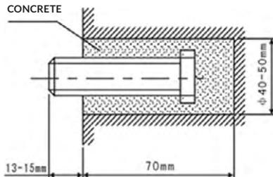
**3.1.3** When the cement has freeze, fit the mounting plate (use the washer and nut according to the following).
