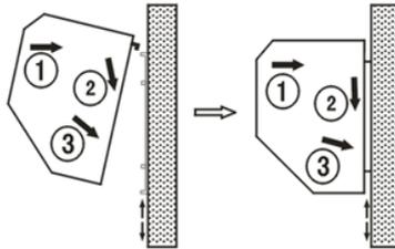
**3.2 Installing on the wooden wall:**
